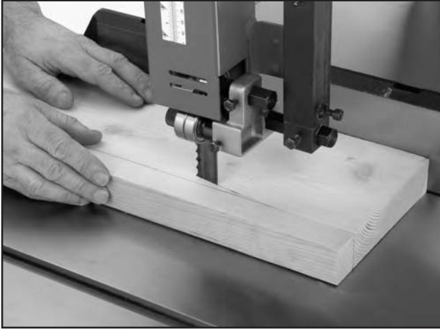
Figure 35. Blade leading away from line of cut.
